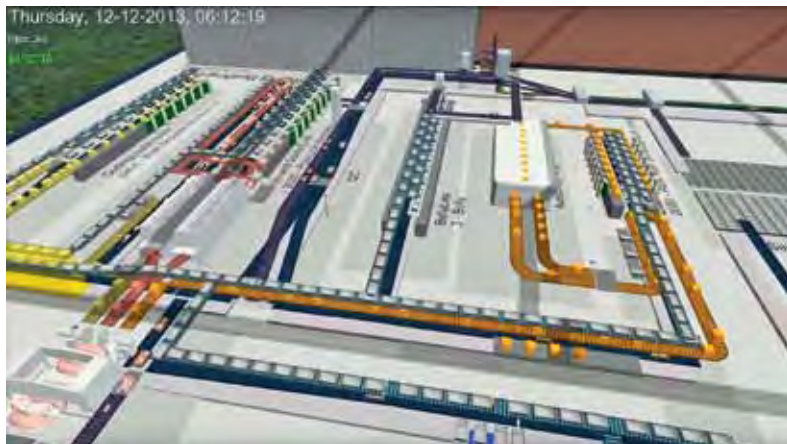
ALECTIA delivers simulation and logistics solutions for businesses in the process industry. This image shows a simulation where ALECTIA has used FlexSim to model the flows and processes of a slaughterhouse. Find the full simulation video on YouTube – search for “Alectia food processing simulation”.
