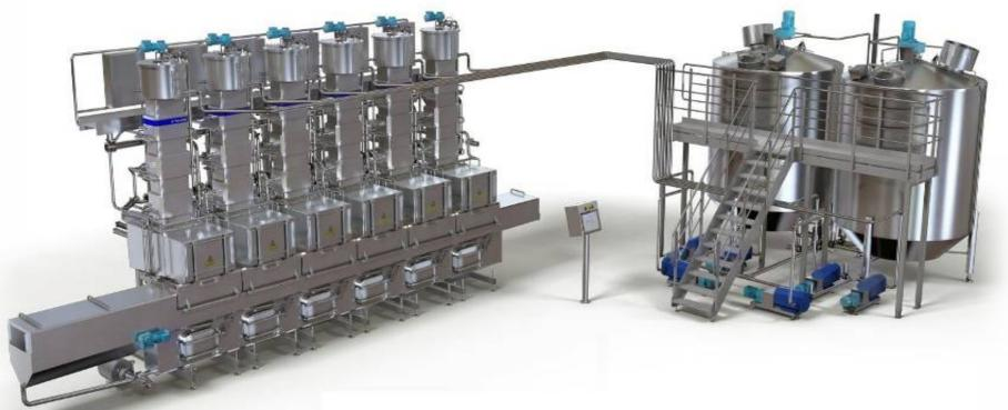
Continuous whey drainage and portioning machine for efficient semi hard and hard cheese for 1 cheese size
